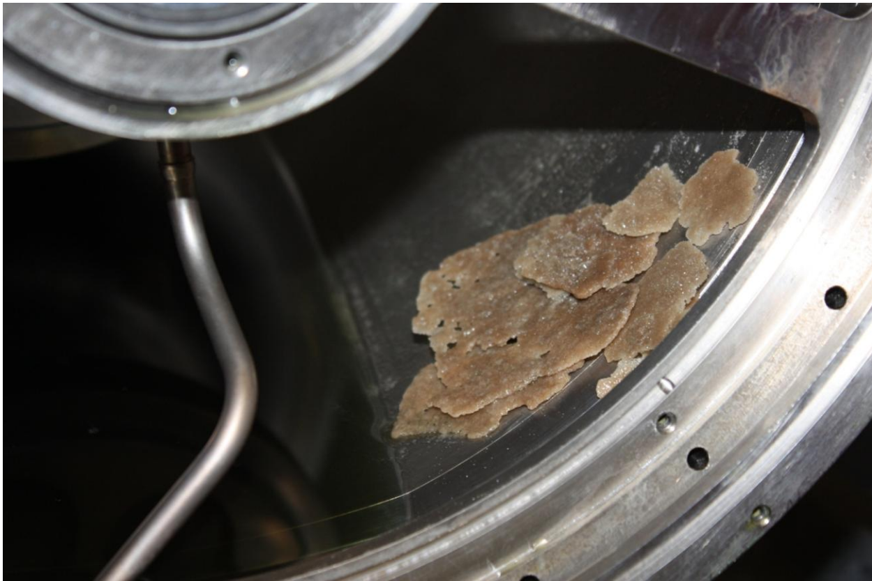
Figure 6. Precipitation in the Distillation Assembly Evaporator
