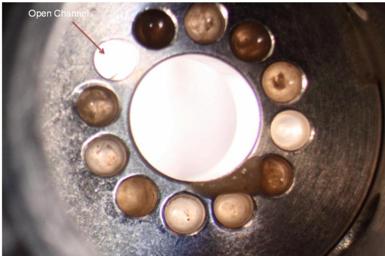
Figure 7. Biomass Present in MLS Inlet Solenoid Valve
