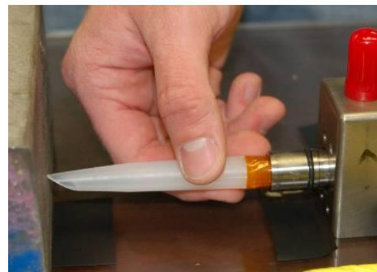
Figure 5. Removal of Check Valve (ground demo)
