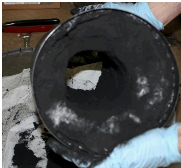
Figure 12. Carbon Brick from H-Bosch. Carbon formed on shredded steel wool within a H-Bosch cartridge. The center and ends of the cartridge have been removed to show the structure of the brick. The white area is insulation embedded with carbon.
