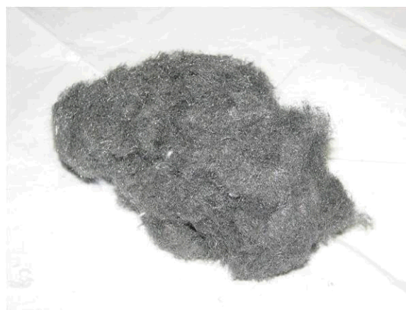
Figure 4. Shredded Steel Wool. Shredded steel wool was used in both Bosch Baseline and Alternative Catalyst Testing.
