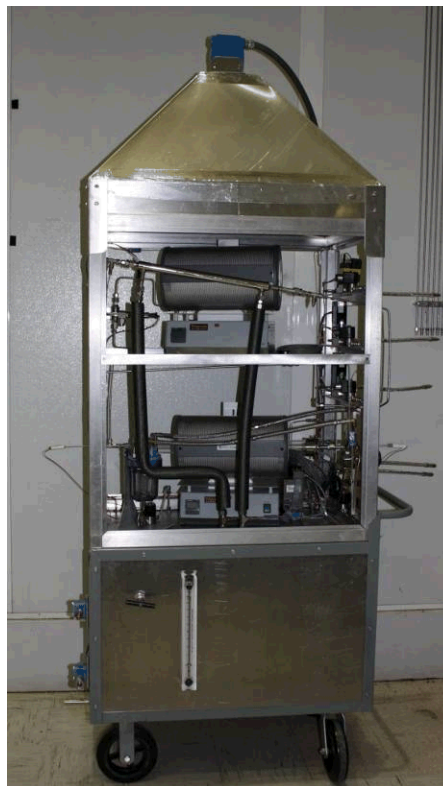
Figure 2. Bosch Catalyst Test Stand. The B-CaTS provides a quartz reactor in a tube furnace for Bosch catalyst testing.
