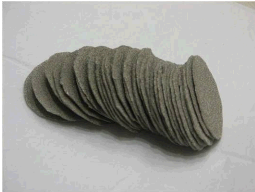
Figure 6. Nickel Foam Catalyst. Nickel foam was cut into 4.5 cm disks for testing.
