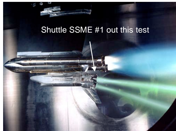
Figure 37. Space Shuttle Aerodynamic/Propulsion Model Tests at AEDC and at NASA/Lewis
