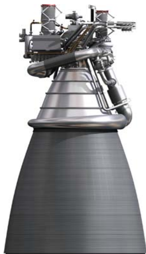
Figure 9. J-2X Engine to be installed in SSC Test Stand A3
