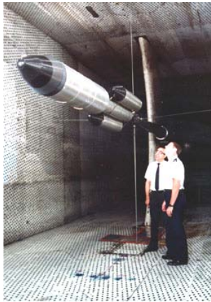
Figure 29. The Titan IIIC Launch Vehicle in the AEDC 16-Ft Supersonic Wind Tunnel and Titan IV in the 16-Ft Transonic Wind Tunnel
