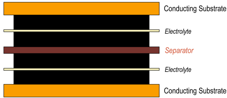
Figure 3. Generic super-capacitor schematic.
