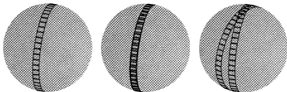
Fig. 3.— Cartoon showing WISE coverage on the sphere for 1 orbit, for 2 consecutive orbits, and for 2 orbits separated by 20 days, illustrating the highly redundant coverage at the ecliptic poles.
