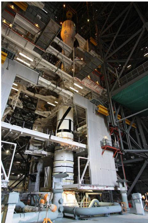
Figure 3. The Ares I-X first stage and new forward structures stacked in the Vehicle Assembly Building
