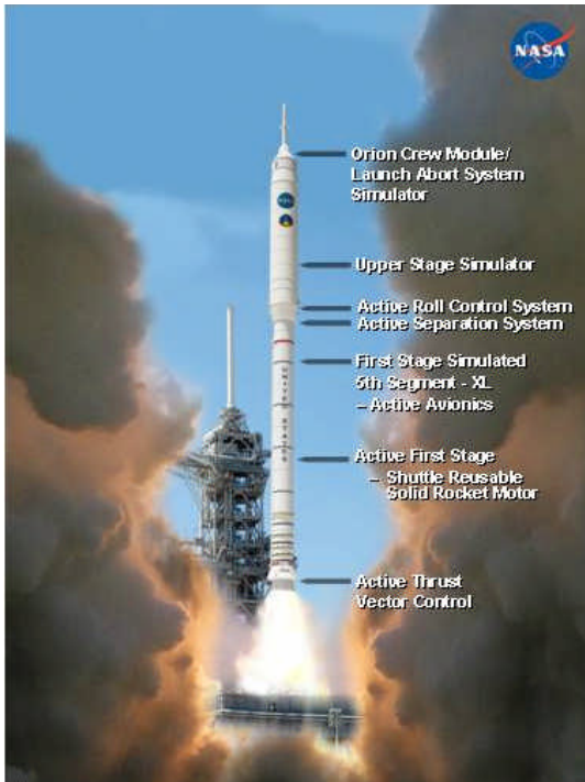
Figure 1. The Ares I-X Flight Test Vehicle incorporates both flight-like and mass simulator hardware.
