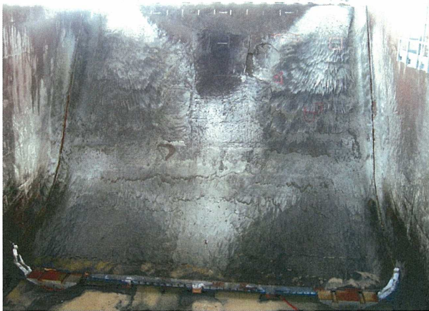
Figure 2. SRB MFD. The light areas at the top left and right are the direct impingement areas.
