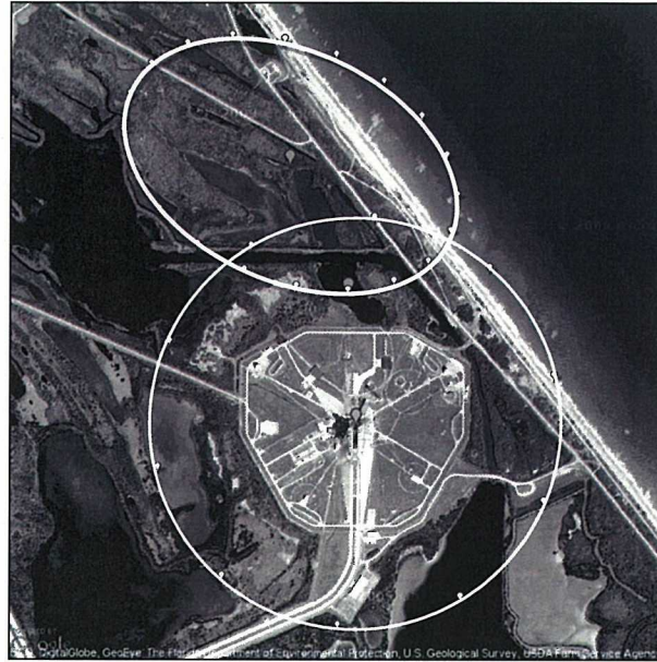
FIG. 13. Google Maps visualization of the 99% confidence uncertainty ellipse for a lightning strike near Complex 39A on 03 August 2009. Figure 13 shows a probability of 6.4% of the lightning strike occurring within the 0.45 nmi radius.
