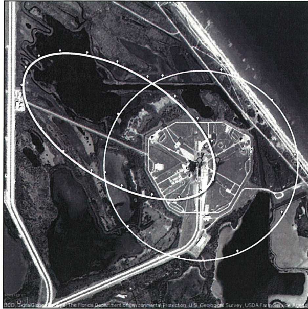
FIG. 11. Google Maps visualization of the 99% confidence uncertainty ellipse for one of the closest lightning strikes to Complex 39A on 03 August 2009. The center of the ellipse was within the 0.45 nmi radius. There is a 54.4% probability that the lightning occurred within that radius.
