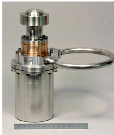
Figure 7.—Sunpower, Inc. thermoacoustic Stirling convertor. Image courtesy of Sunpower, Inc.
