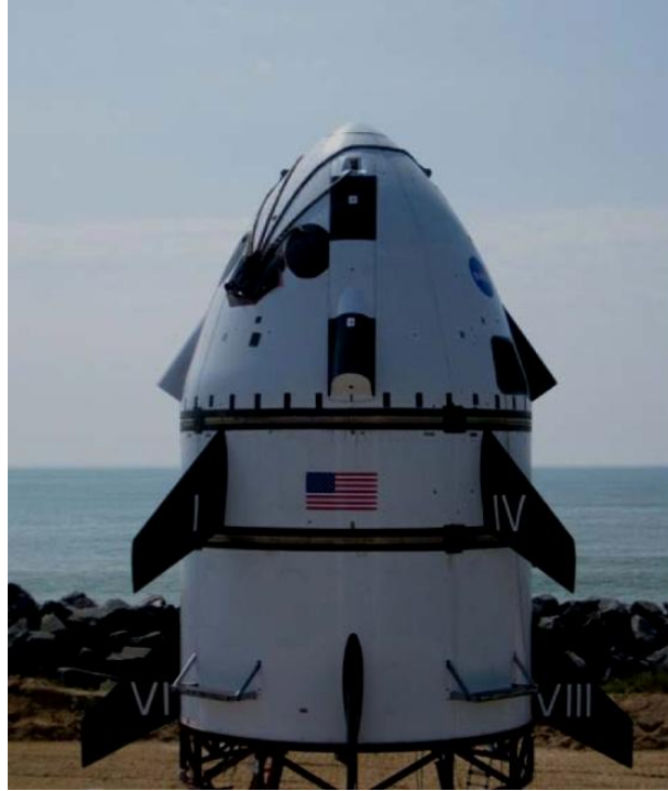
Figure 4. MLAS FTV on launch stool at Wallops Island.
