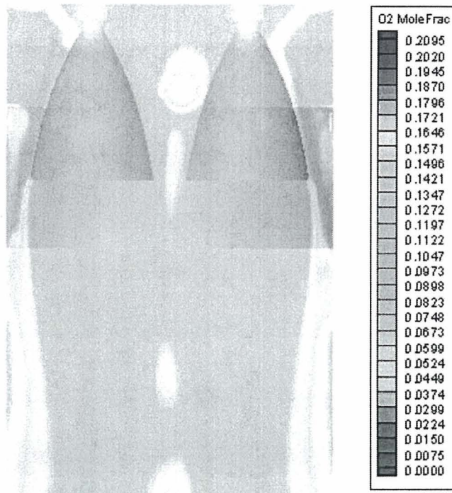
Fig 20 O2 mole fraction at the symmetry plane
