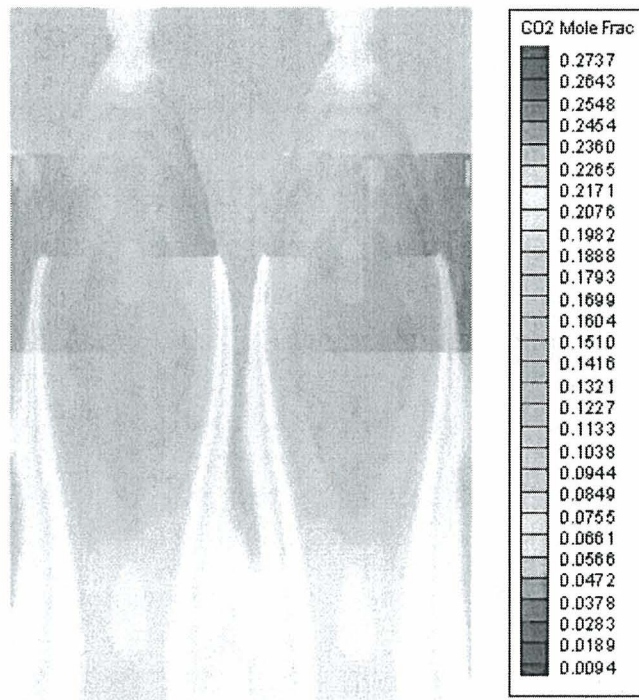
Fig 17 CO2 mole fraction at the symmetry plane
