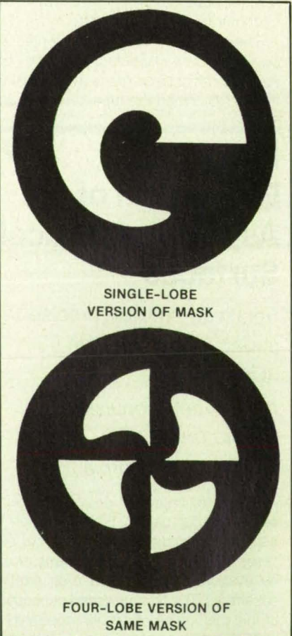
Figure 2. Multiple Lobes reduce the sensitivity of the deposited surface profile to decentration of the mask.
