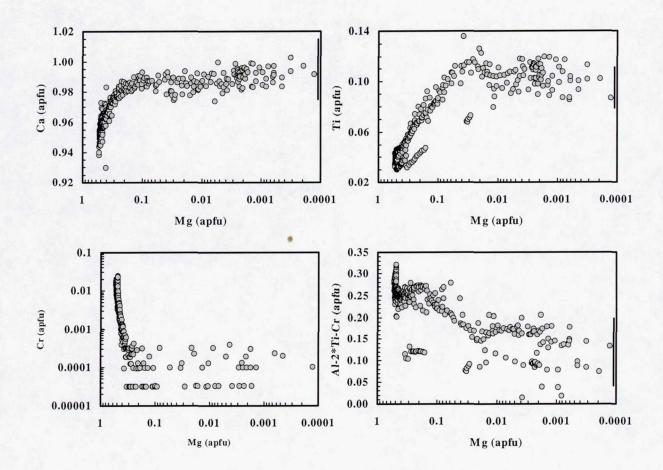
Figure 6. Variation of Ca, Ti, Cr and Al-2\*Ti-Cr, Ti with Mg (all in atoms per formula unit) for clinopyroxene. Vertical bars show ranges in compositions for analyses with Mg of 0 apfu. The wide range in Ca at Mg ~0 is due to P-rich clinopyroxene in rim areas intergrown with silico-phosphate. Note that some analyses are distinct in both Ti and Al-2\*Ti-Cr.
