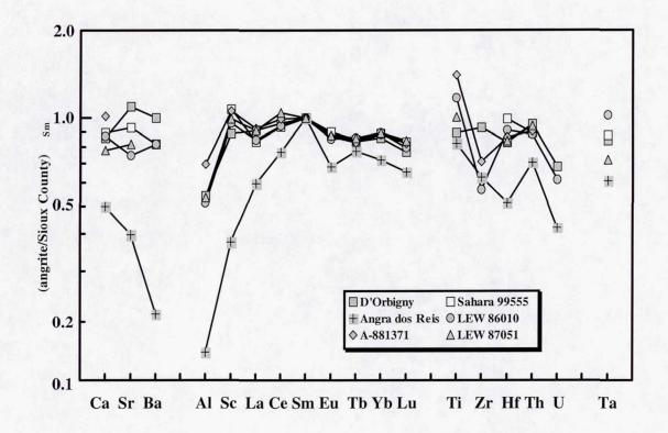
Figure 11. Sioux County- and Sm-normalized incompatible element contents of angrites plotted in order of increasing valence and Z. Data are from the sources listed in Fig. 10, plus Tera *et al.* (1970), Wasserburg *et al.* (1977) and Yanai (1994). Sioux County average calculated from a database of all available literature data.
