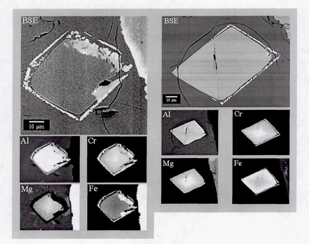
Figure 9. Back-scattered electron images and element maps of euhedral hercynitic spinel grains enclosed in clinopyroxene (left) and plagioclase (right). Note elemental zoning over a scale of a few  $\mu$ m, and Cr-rich rims.
