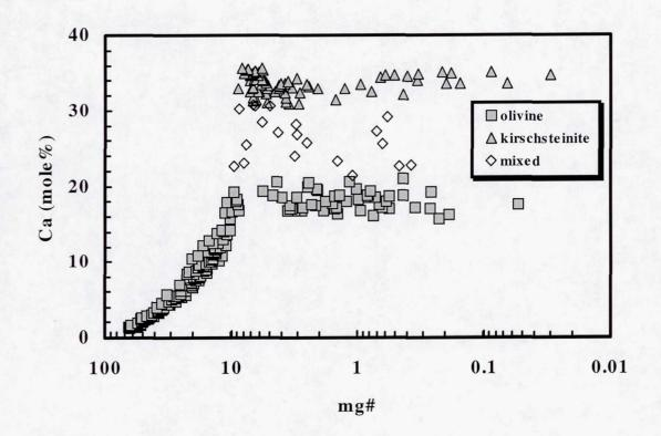
Figure 3. Ca (mole%) *vs.* mg# for olivine and subcalcic kirschsteinite in D'Orbigny. Open symbols (mixed) indicate analyses we believe overlapped both phases. Note distinct gap in olivine compositions between about mg# 9 and 6.
