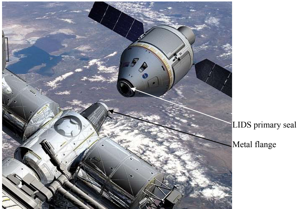
Figure 2.—Drawing of a manned capsule docking with ISS; LIDS enables the coupling of the two together; the elastomer of the LIDS primary seal stops air from leaking out after docking.
