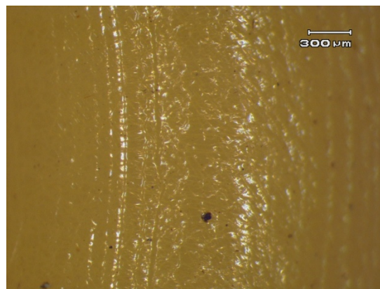
Figure 16.—Esterline size #2-309 o-ring after atomic oxygen fluence exposure of 5.7 \times 10^{21} atoms/cm 2 and UV exposures of about 1170 ESH in the VUV/NUV ranges.
