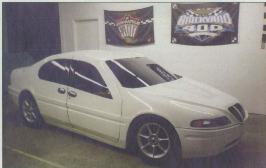
Photo 5: The Paradigm™ prototype car makes extensive use of acrylic coated plastic body panels.
