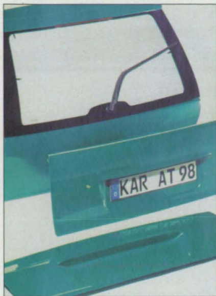
Photo 3: An even greater use of plastics in automobiles is large parts such as rear hatch panels.
