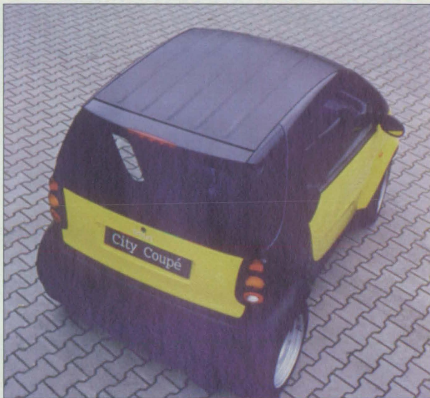
Photo 4: The new Smart Cars from Mercedes incorporate a plastic one-piece roof and roof liner.
