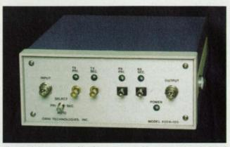
Fiber-Optic Transceivers like this one are used in pairs to transmit digital signals from remote test locations at rates up to 125 Mb/s. Whereas the maximum usable length of a coaxial cable for transmission of analog signals in the original application is 50 m, the maximum length of a fiberoptic digital link in the same application is 25 km.
