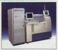
Hewlett-Packard, Palo Alto, CA, has introduced the HP 4072A semiconductor test system for process verification of next-generation CMOS (Complementary Metal Oxide Semiconductor) integrated circuits at high throughput. The parametric system also provides Flash memory-testing capability, rapid wafer level relia-
