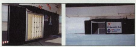
Figure 2. Specimens of Exposed Materials from the X-33 launch vehicle and the external tank of the space shuttle were mounted on the carrier plate of the flight-test fixture.
