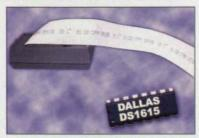
Dallas Semiconductor, Dallas, TX, offers the DS1615 one-chip instrument for measuring temperature integrity and variability over time. The chip integrates a Y2K-compatible real-time clock, digital thermometer, control logic, serial interface,
