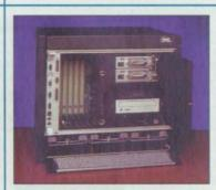
The Model CP8000 CompactPCI rackmount enclosure from SBS Technologies, Vista, CA, features hot-swappable power supplies and fans. The 9U high enclosure comes standard with an 8-slot CompactPCI backplane for 6U cards, and can accept special telephony backplanes. It also accepts a variety of plug-in CompactPCI
