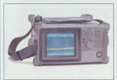
Tektronix, Beaverton, OR, offers the U3661 portable spectrum analyzer, a 26.5-GHz instrument for field installation applications. The unit weighs 24 pounds with batteries and spans the frequency range of 9 kHz
