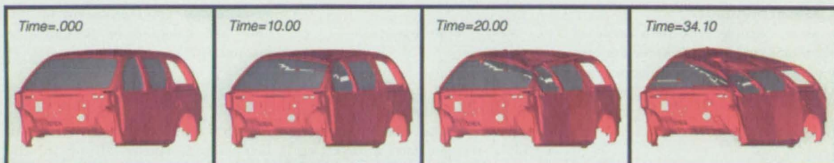
Rollover analysis of a minivan produced by the ADINA System. The simulation shows the result of a rigid surface (representing a road) being pushed against the van at a very slow speed.
