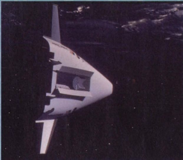
The X-33 will launch vertically like a rocket and land horizontally like a plane.
