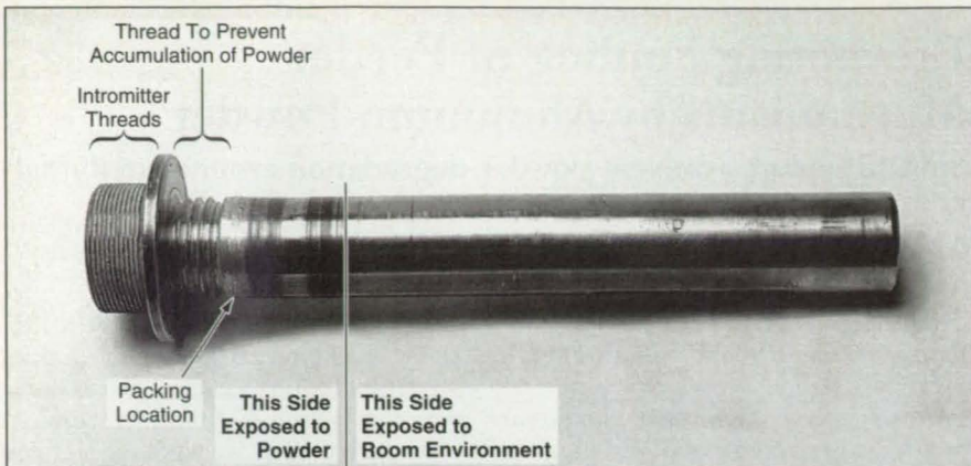
The Deep Thread just to the right of the flange acts as an auger to prevent the accumulation of powder inside the hopper near the packing seal.
