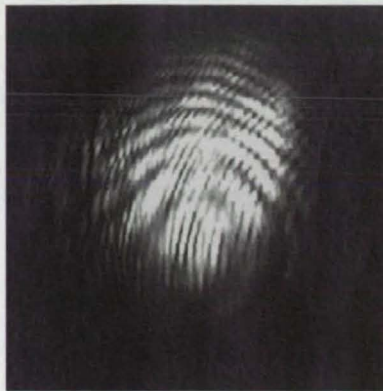
INTERFERENCE PATTERN FORMED FROM PHASE-CONJUGATE RETURN OF ABERRATED BEAM
