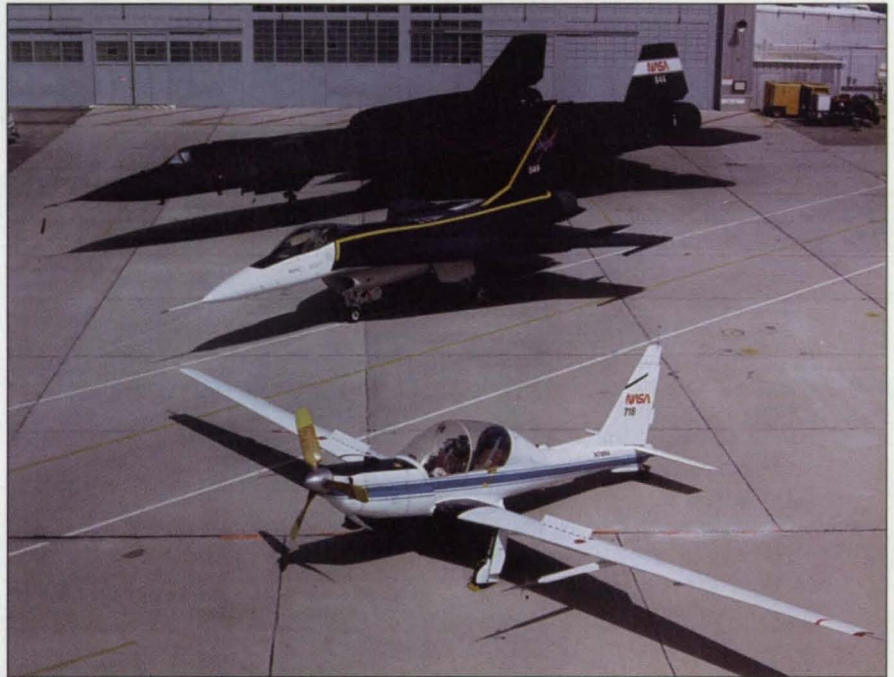
Figure 1. These Airplanes Were Used to gather data on sonic booms. From top to bottom, they are the SR-71, F-16XL, and YO-3A.
