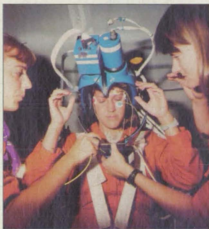
Incorporating optokinetic modules and accelerometers, this helmet will study space adaptation syndrome on the first In-Flight Medical Laboratory. Other state-of-the-art sensor technologies are described in our feature story, beginning on page 8.
