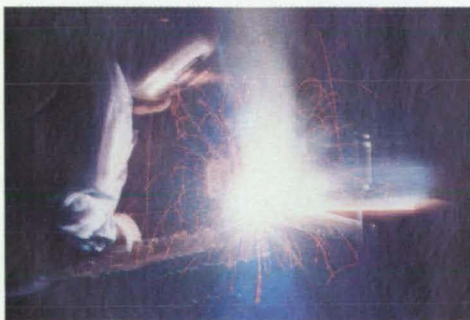
During processing, beryllium material is welded into a steel can prior to being rolled into a sheet. Used wherever light and stiff metals are called for, metallic beryllium is produced by Brush Wellman, of Cleveland, OH. (Photo courtesy Brush Wellman).
