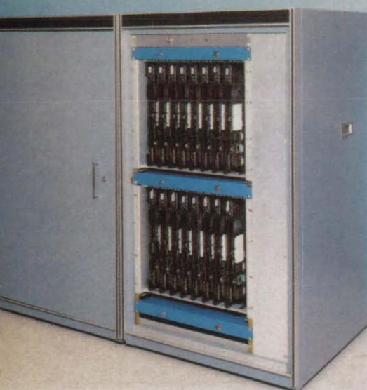
This 32-node Mark III Hypercube has the computing power of 32 to 64 of the VAX 11/780 minicomputers.
