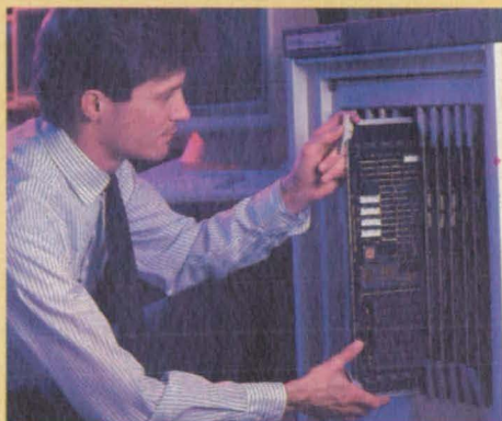
The Series 1200 configured with 8 super minicomputers and 17 mb of static memory (SRAM).
