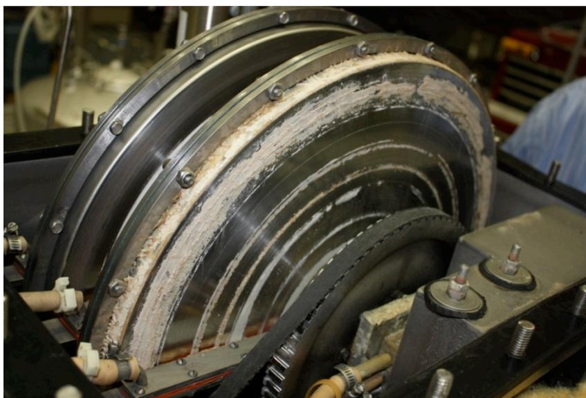
Figure 4. Precipitation of solids on disks at end of test.
