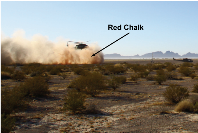
Figure 24. View from Camera 2 of Lane 7 approach to touchdown event with red chalk pickup visible
