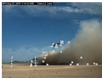
Figure 14. Brownout cloud analysis from first round of testing, Lane 7 approach to touchdown
