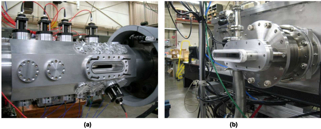
Figure 1: (a) EAST test section showing slot window primary. (b) Slot window secondary
