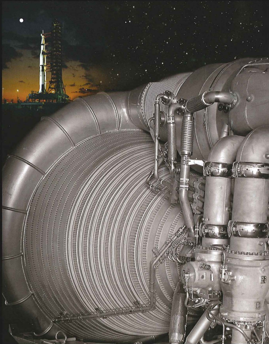
An F-1 engine fueled by oxygen and kerosene; five F-1's powered the Saturn V first stage of the Apollo launch vehicle.
