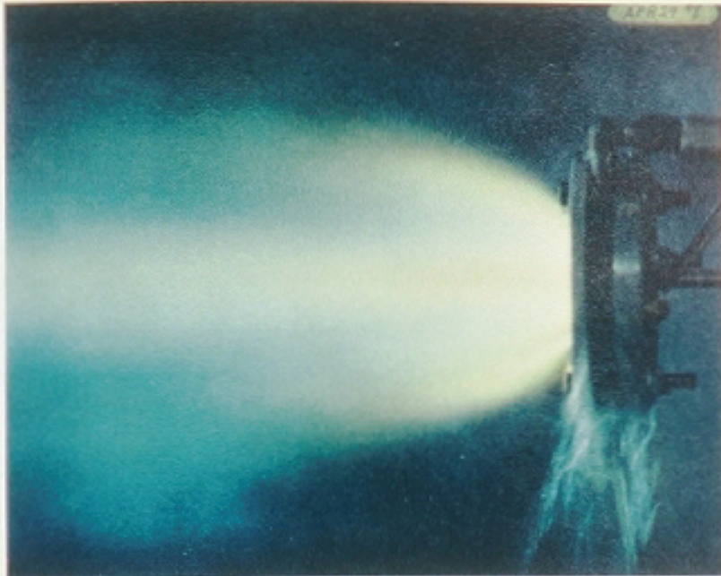
Plate 26. Concentric-Tube Injector of Plate 25 with 0.15-in.-long Chamber
