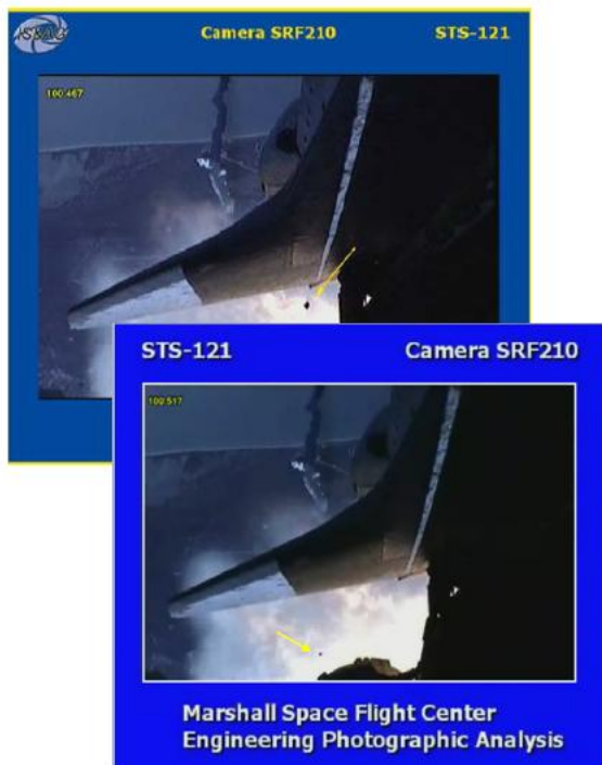
Figure 6. STS-121 ascent imagery of foam debris liberated from the Space Shuttle ET. (cf. Reference 7).
