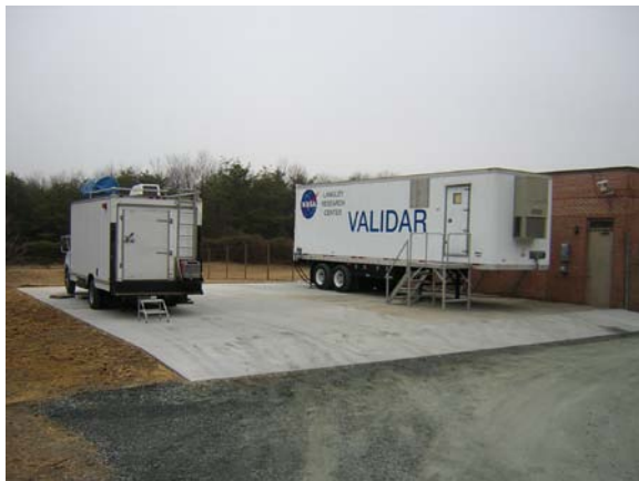
Fig. 2. Photograph of field test site at the Howard University Research Campus in Beltsville, Maryland. The 2- \mu m lidar is housed within a 35-foot long trailer testbed called VALIDAR. The other trailer houses the Goddard Lidar Observatory for Wind.
