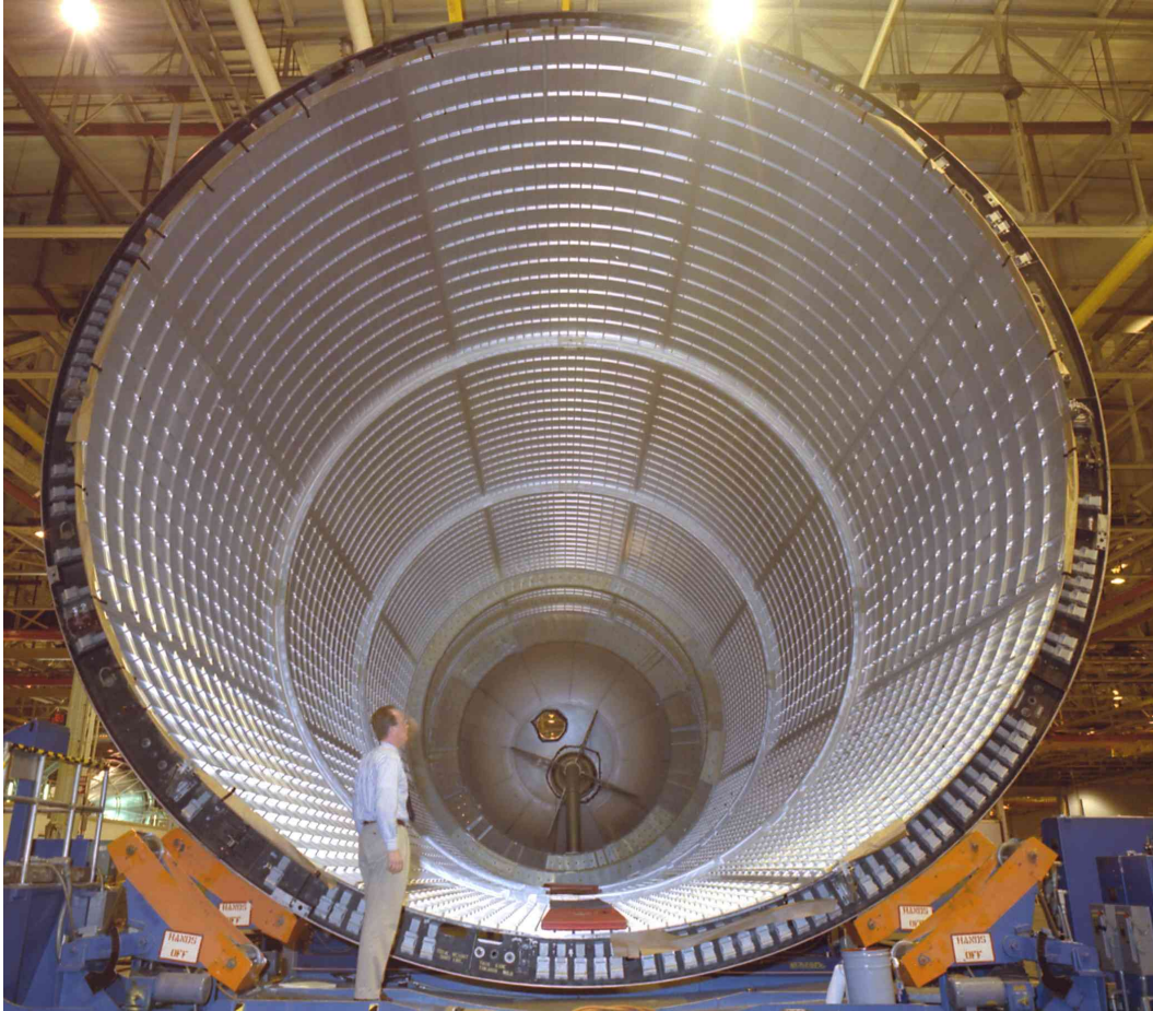
Figure 4. SLWT LH 2 tank barrel assembly (Lockheed Martin photo).
