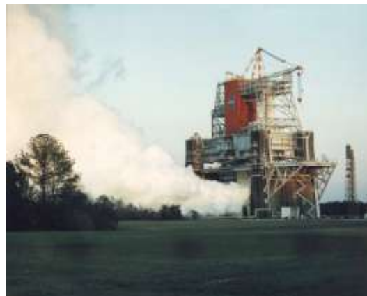
Figure 1: Space Shuttle Main Engine Test at the NASA Stennis B-1 Test Stand.
