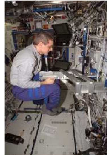
Expedition 12 crewmember Bill McArthur activating the SLAMMD in the HRF 2 rack
