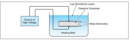
A **Polymer Substrate Is Heated** to its softening temperature in a low-permittivity dielectric liquid while a high voltage is applied to metal electrodes on opposite faces to induce electric polarization. When the electrode/substrate/electrode sandwich is cooled, the polarization remains frozen into the substrate.
