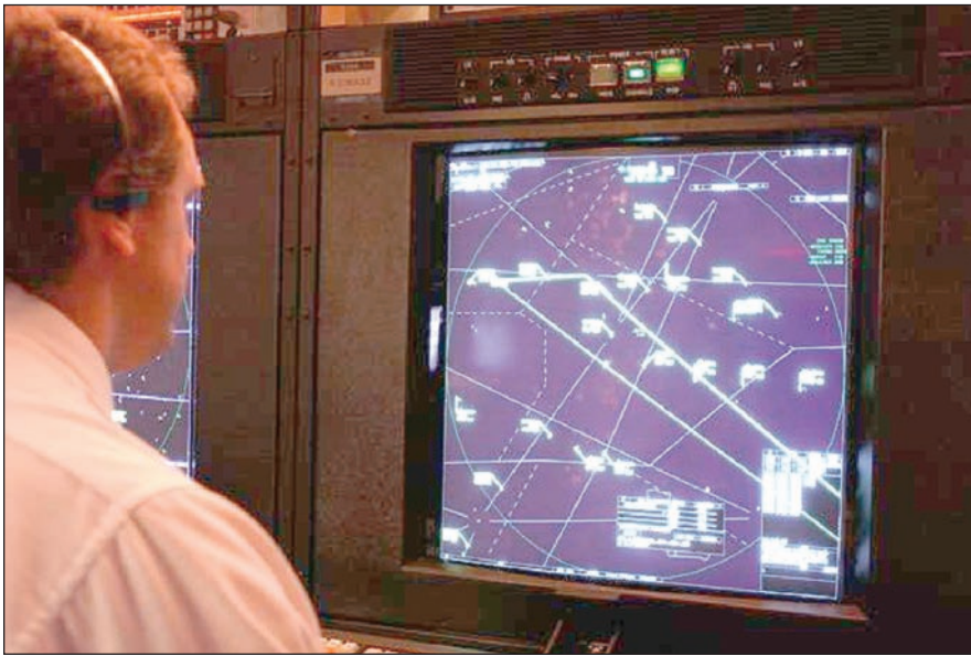
Figure 2. This Display helps the controller identify and work with the highest-pay-off aircraft.
