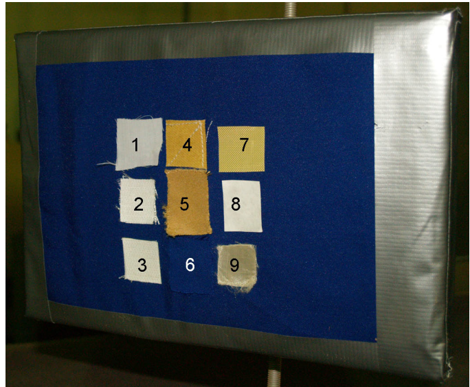
Figure 2. Fabric samples for the Martian pressures tests in the MARSWIT. (1) Apollo-era FEP, (2) Orthofabric, (3) silicone backed Orthofabric, (4) NDX2OL, (5) NDX1RL, (6) NDX1OL, (7) silicone backed Kevlar, (8) Tyvek, and (9) silicone backed Vectran.
