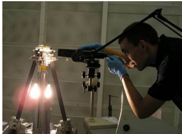
Summer student Kyle Norman uses a camera to inspect a bond during construction of the silicon carbide telescope structure.
