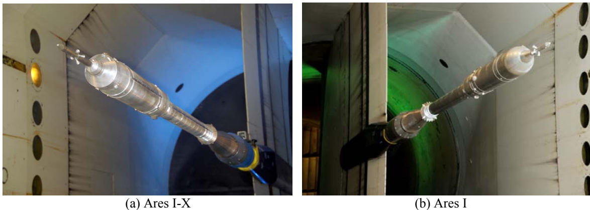
Figure 1. Rigid Buffet Models installed in the TDT test section.
