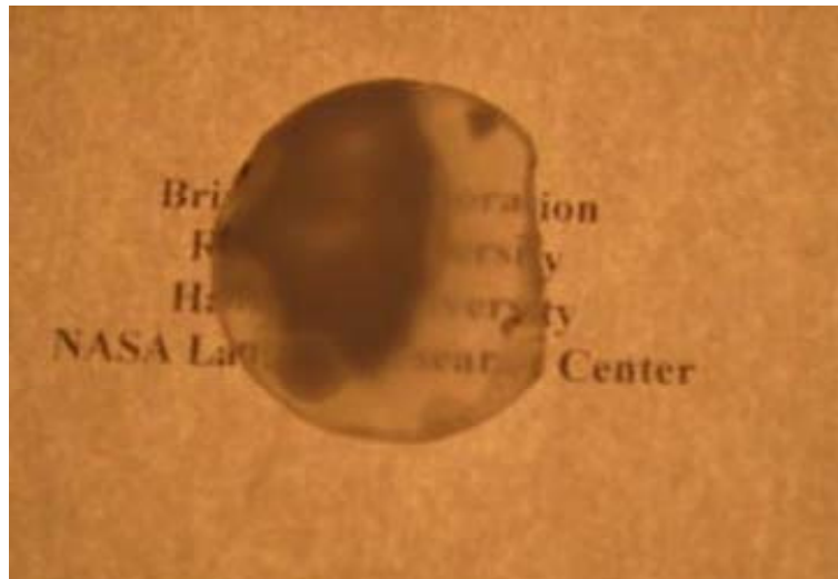
Fig. 9. Ceramic Yttria sample of 2" in diameter with dark regions due to oxygen loss.
