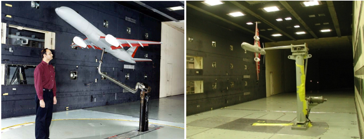
Figure 3. Generic Transport Model (GTM) in the NASA Langley 14- by 22-Foot Low-Speed Tunnel. Left – static mount, Right – pitch oscillation mount.
