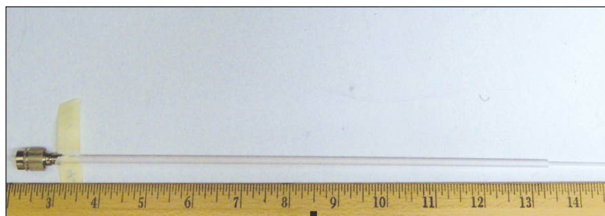
Figure 1. A Probe packaged and connectorized with a fiber Bragg grating (FBG) inside. The FBG is located at the end of the probe inside a smaller-diameter ceramic tube.
