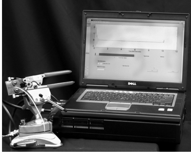
Figure 3: Photograph of the crimp tool data experimental setup.
