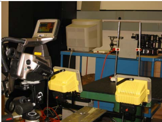
Figure 9. Imaging Damaged RCC Under Simulated Solar Conditions
