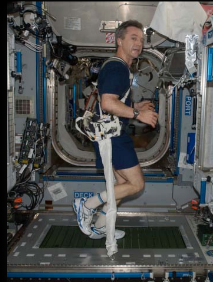
Glenn Harness tested by crewmember on T2 Treadmill during ISS Exp. 21
