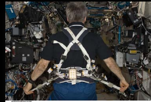
Glenn Harness Back view showing load sensors and Instrumentation
