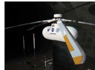
Full-scale helicopter smart blade in a Ames Res. Ctr. wind tunnel
