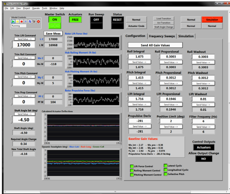
Figure 2: Trim Controller operator interface written in National Instruments Labview.
