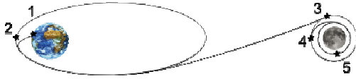
Figure 4: Mission scenario for lunar orbiter, showing the launch into the phasing loops (1) with a C_3 of -2.6 \text{ km}^2/\text{s}^2 , the transfer trajectory insertion (2) with a \Delta v of 50 \text{ m/s} that includes 20 \text{ m/s} for the midcourse correction, the insertion into the lunar checkout orbit (3) with 800 \text{ m/s} , the Hohmann transfer from the checkout into the science orbit (4) with 80 \text{ m/s} , and the orbit maintenance and reaction wheel desaturation maneuvers (5) on the science orbit.
