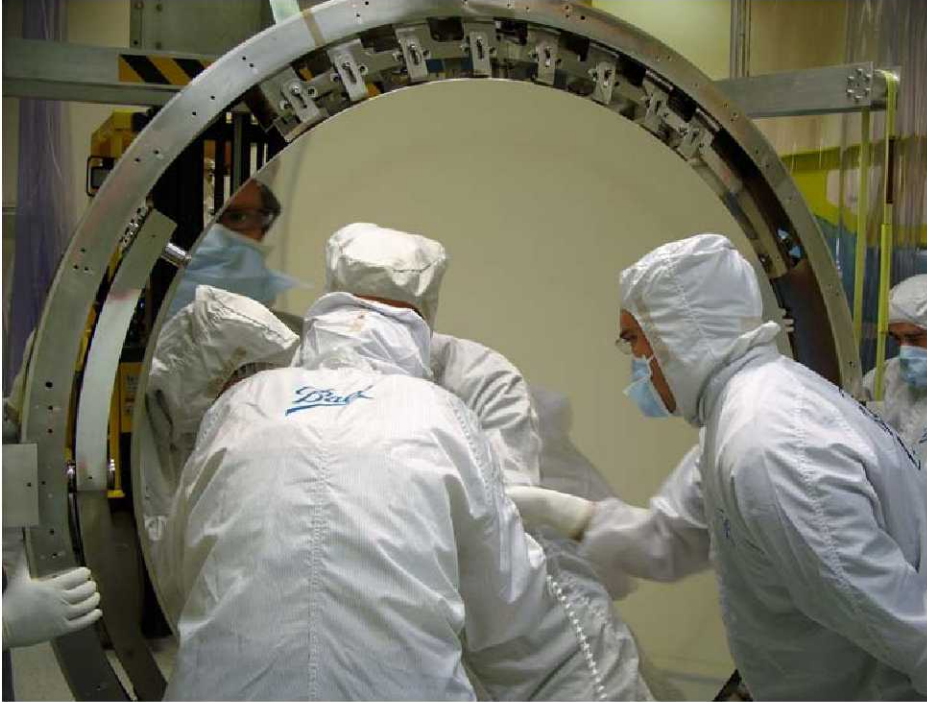
Figure 9 Kepler primary mirror inspection after enhanced silver coating. (Source: Brashear)
