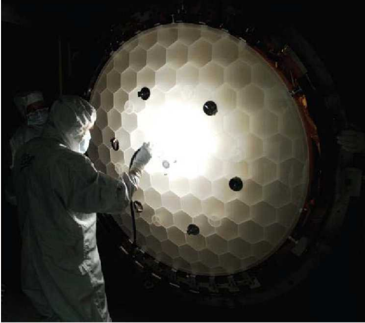
Figure 4 Kepler primary mirror (rear side inspection). (Source: NASA press kit. ://kepler.nasa.gov/pdf files/314125main Kepler presskit 2-19 smfile.pdf )
