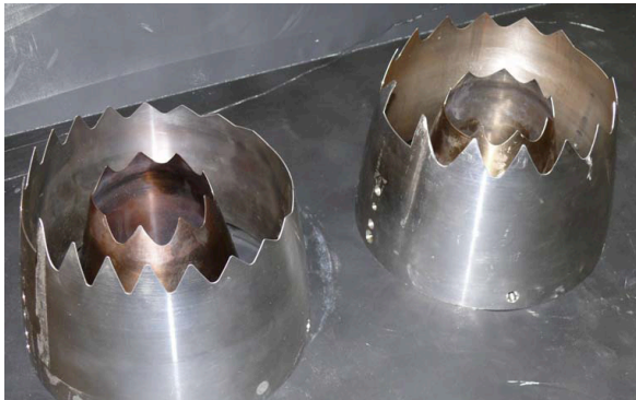
Figure 8. Model scale chevron nozzles, baseline chevron (Chev1, left) and aggressive chevron (Chev2, right).
