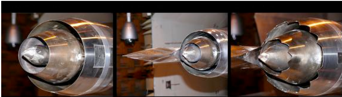
Figure 7: Nozzle configurations, a. LBPR axisymmetric, b. HBPR with pylon, c. Chev2 chevron nozzle.
