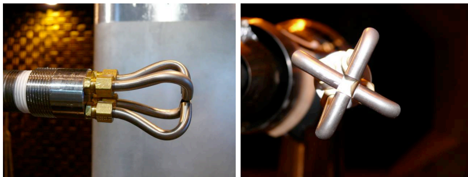
Figure 11. Close-up photograph of impinging jet noise source used as an omnidirectional, point noise source.
