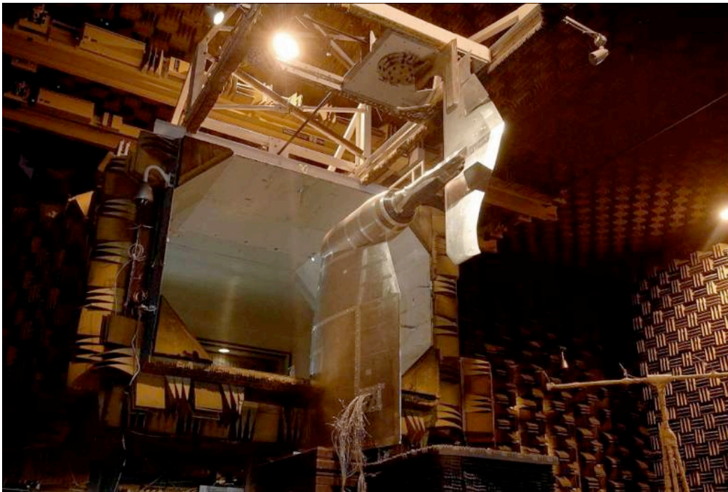
Figure 3. Boeing Low Speed Aeroacoustic Facility configuration for the BWB PAA experiment with the simulated BWB airframe model.
