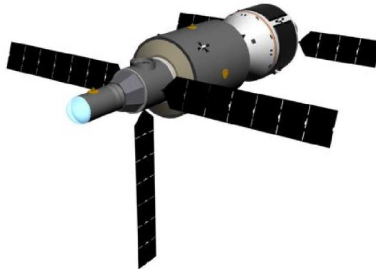
Figure 1. The Flexible Path vehicle for asteroid missions includes an ISS derived habitat and the Orion crew exploration vehicle.
